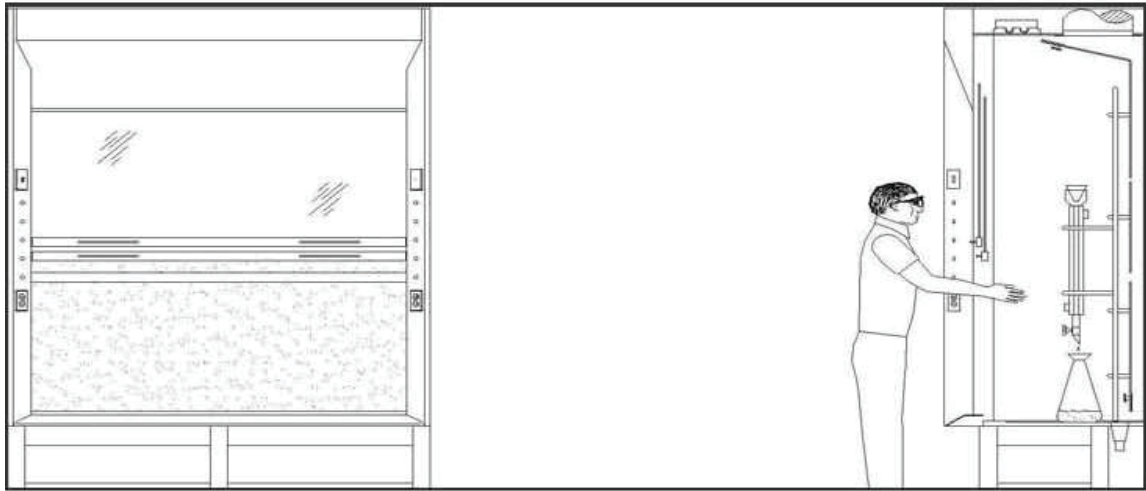
Fig. 7 Typical View of Distillation Fume Hood
