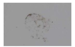
Level 3 (Etch, Pitting, Cratering, swelling or erosion of surface)
